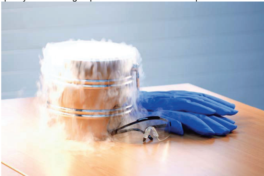
Liquid nitrogen “boiling” at room temperature (Courtesy AGA)
