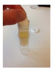
Without touching the gel put the Dip Slide into the tube
