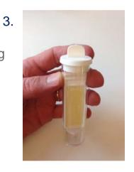
Keep the Dip Slide warm (min. 37° C) for 48 h.
