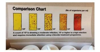
If bacteria is present in the Cooling Water , red spots will show on the Dip Slide Gel
