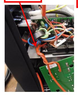
Keep up the wire (it must not be close the power board)
