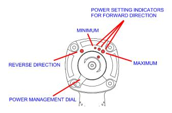
The Impact wrench incorporates a Power Management System that allows the operator to select 3 power output settings. These settings range from minimum power output through maximum power output in the forward direction only.
