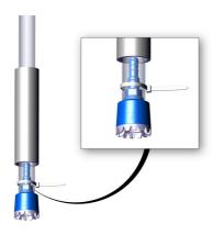
Cable tie the clear PVC chemical suction tubes. Once the tubes has been connected and sealed securely in place, attach the foot filter along with the ceramic weights and place in receptacle.
