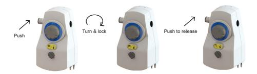
The High Flow system has an automatic locking feature to continually dispense diluted chemical. To activate the feature, remove the plug with the small lock symbol and push and turn the grey operating button clockwise. When the container is full, simply push the operating button again to deactivate. Once the system has been set up for high or low flow application, replace cover and attach the water main to inlet.
