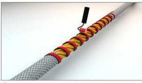
**Step 4** Wrape the polyester cloth around the taped, damaged area.
