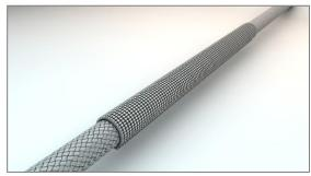
**Step 9**Complete the repair using the white vinyl tape to cover the vulcanized tape.
