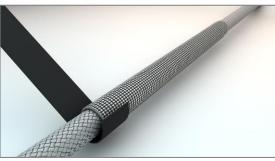
**Step 10**Use white seizing rope on top of the white vinyl tape, in addition to each 50 cm between the taped areas for optimal safety and fit.
