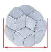
Rope diameter: "M" size 38mm - 54mm "S" size 24mm - 36mm
