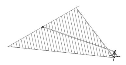
The safety zone for the operation is designated as a 60° triangle with a top point at the center of the tripod. This area must be clear of personnel while the product hanging in the wires.
