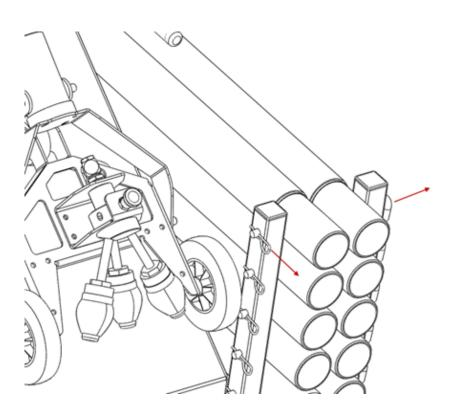
Unload all Tubes by removing lock pin
