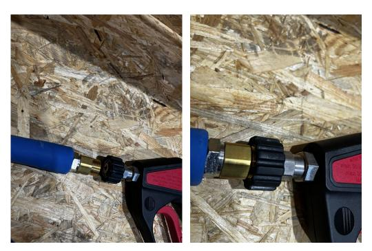
From the trigger gun, connect one more blue extension hose, with the male M22 and either extend same with one more hose, or connect this directly to the Navadan Tool Carrier Head as shown above.
