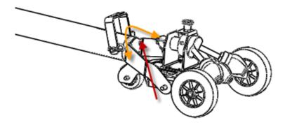
If needed, adjust the tilt of tool carrier (both front wheels to touch the surface) with 4X Unbraco screws.
