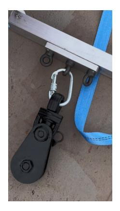
Snatch block should be attached to the aluminium carriage like this.
