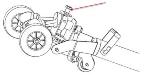
Adjustment for flat surface or frame cleaning by tilting nozzles.
