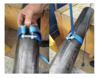
Screw the bolt back onto the D-shackle (18) and pull the webbing (15/16) to make the loop tight.
