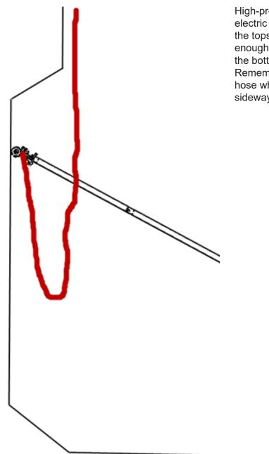
High-pressure hose and electric cable hung from the topside with just enough length to reach the bottom of the tank. Remember to move the hose when changing position sideways.
