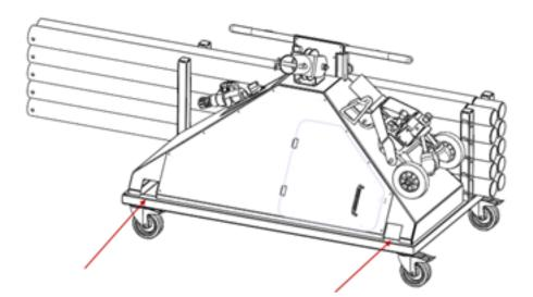
Attach sling set to lifting points (4 Pcs) and hoist unit into the cargo hold.
