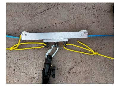
The two oguide ropes(6mm yellow or white lines) attached to either side as they are for lateral movement of the aluminium carriage on the webbing. These two guide ropes are to be placed over the hatch coaming on deck in order to move and secure the carriage.
