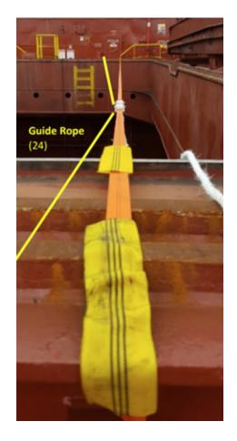
GUARD AGAINST WEAR from sharp edges using the Webbing Protector sleeves (17) where appropriate
