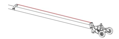
Mount tool carrier at end of the tube (see picture on next page) Mount wire bracket at last 2 pins before tool carrier. (To reach under a large overhang, move the wire bracket to pin 2 and 3 from the tool carrier instead of 1 and 2).
