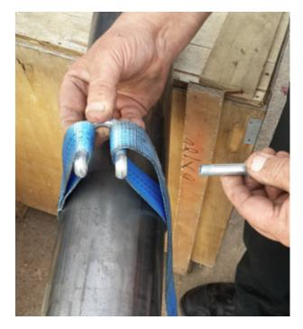
Undo the D-shackle (18) then feed through the end loop and around the webbing to create a loop like so.
