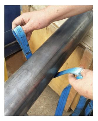
Fixed end of line. Blue/orange webbing used to make anchor point on ship. Find two horizontal secure poles that are parallel to each other on opposite sides of the cargo hold to attach the webbing (15/16) to. Loop the webbing around a pipe or coaming bracket as shown below.
