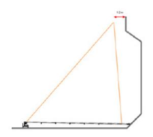
Blue/Orange webbing spanning cargo hold to be placed 1-2 m from the top wall (this is the one which will be going from one side of the cargo hold to another). See the picture below.
