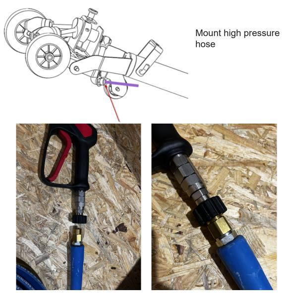
From the high pressure cleaner, connect one of the blue extension hoses (using the female M22). Thereafter connect the male M22 to the trigger gun.
