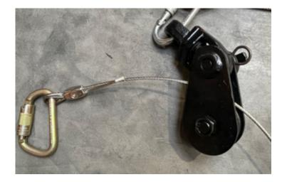
Close the snatch block and lower the wire down to the tool carrier. Adjust Ø5 lines to snatch block. It is located over the tool carrier.
