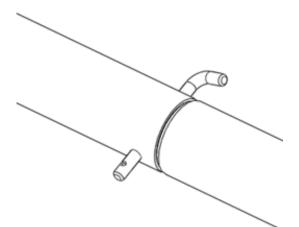
Mount tubes for cleaning height + minimum 2m. Mount short pin for locking tubes – do NOT mount split.\* Pins are located in the compartment of the base unit.
