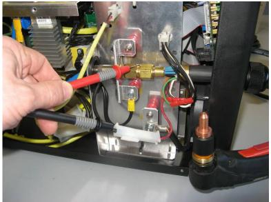
Remove shield cup body and repeat the measure between Current/air lead and pilot connector.
