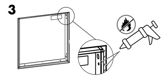
Gaps between El60 box and walls, and screw recesses to be filled with fire retardant sealant.
