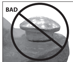
Oval Neck of Bolt Not Seated Properly
