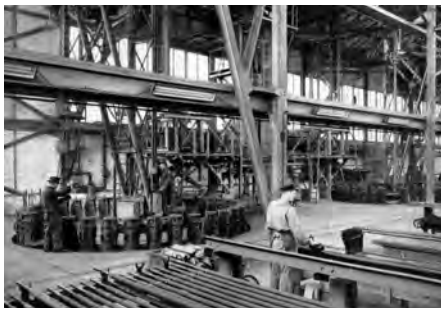
Carousel carrying upright sand moulds of about 1900
