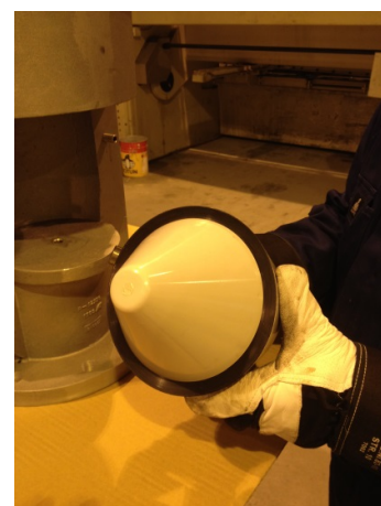
Check gasket on float
