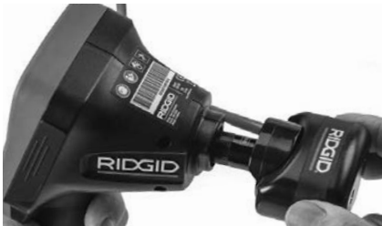
Figur 18 – Kameraets tilkopplingsplugg installert
