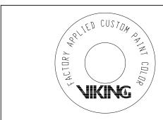
Identification of Custom Paint Color: All custom color painted cover plates will have an identifying label affixed to the inside of the cover that indicates custom color and will have a representative sample (a paint dot) of the paint on the label.
