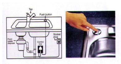
Air switch is available for every models and offers additional ease of installation and usage. The button of the accessory can be located on the work top or sink. The button can be located on the work top or sink. Pressing the button sends a pulse of air through a tube the disposer to switch it on and off. The air switch is supplied with interchangeable white and chrome finishes.
