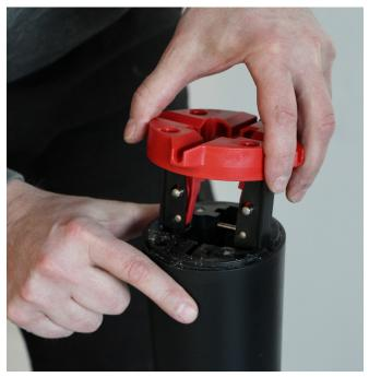
01 / Remove fixating. 02 / Place new. 03 / Tighten. 04 / Ready for use
