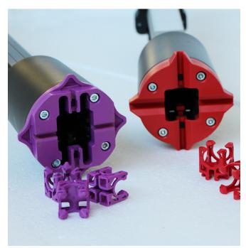
Make sure that the colour of the fixation is the same as the colour of the clip.
