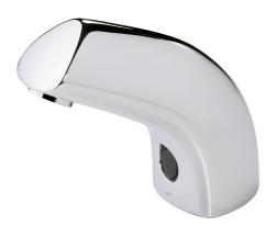
Touchless washbasin faucet with a mixing valve. Fixed electrical connection 230 V. Recognition range can be adjusted at the faucet. The faucet is equipped with litter filters and non-return valves.
