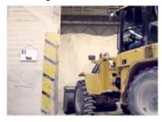
Mineral raw materials (clay, kaolin, feldspar and silica) are unloaded from trucks in the areas marked for this purpose.
