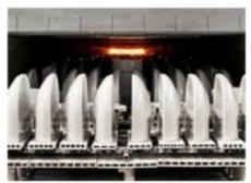
The enamelled pieces are then transported to the kiln area for their firing. The process of heating, firing, enamel vitrification and cooling takes place inside the kiln.
