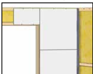
6) Illustrations showing solutions for starting at a door or an inside corner. 6b is only used for 2-pcs inner corner profiles.
