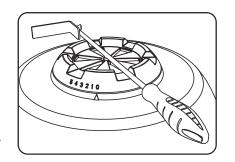
Adjust the dampers using the Multi-Tool.
