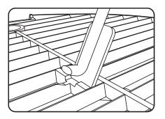
The chrome plated grill grate provides an additional cooking surface. When using the chrome grate, the cast iron grate must be in the lower locked position. The chrome plated cooking grate can swing out of the way to access the lower cooking grate during cooking.
