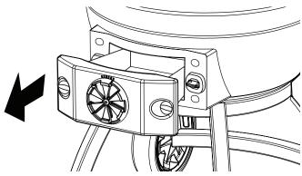
When the charcoal ashes do pile up, remove the charcoal ash catcher. Only perform this when the grill is cool and charcoal has been extinguished.
