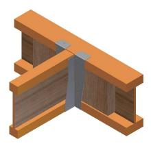
Figure B4 – Enhanced top fix I-joist to I-joist.
