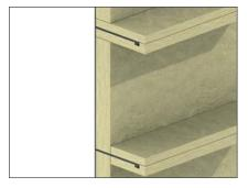
Example of A60 class solution for steel bulkhead with PAROC Marine Fire Slab 100 and preformed block PAROC Marine Fire Slab 100, Pulb. Insulating thickness on bulkhead is 60 mm and on stiffener 25 mm.
