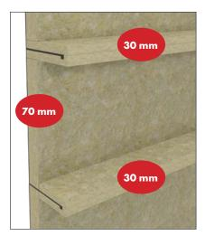
Example of A60 class solution for steel deck with PAROC Marine Navis Slab 60. Insulating thickness on bulkhead is 70 mm and on stiffener 30 mm.
