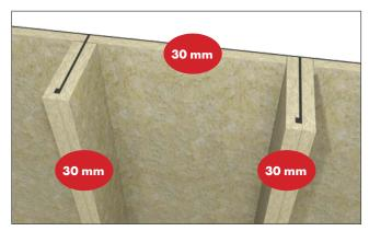
Example of A30 class solution for steel deck with PAROC Marine Navis Slab 60. Insulating thickness on deck and on stiffener is 30 mm.
