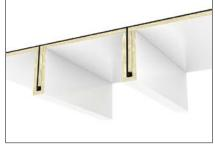
Example of A30 class solution for steel deck with PAROC Marine Fire Slab 100 G1 and preformed block PAROC Marine Fire Slab 100 G1, HPL. Insulating thickness on deck and stiffener is 25 mm.
