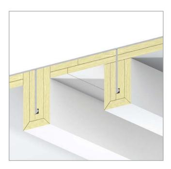
Example of A60 class solution for aluminium deck with PAROC Marine Fire Slab 100 G1 and preformed blocks, insulating thickness is 25 + 25 mm.
