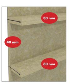
Example of A30 class solution for steel deck with PAROC Marine Navis Slab 60. Insulating thickness on bulkhead is 40 mm and on stiffener 30 mm.
