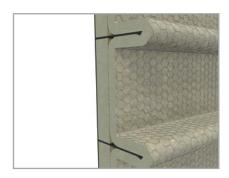
Example of A60 class solution for steel bulkhead with PAROC Marine Wired Mat 100. Insulating thickness on bulkhead is 50+30 mm and on stiffeners 30 mm.
