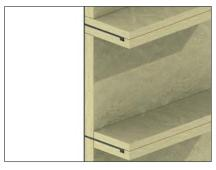
Example of A30 class solution for steel bulkhead with PAROC Marine Fire Slab 100 and preformed block PAROC Marine Fire Slab 100, Pulb. Insulating thickness on bulkhead is 40 mm and on stiffener 25 mm.
