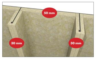
Example of A60 class solution for steel deck with PAROC Marine Navis Slab 60. Insulating thickness on deck is 50 mm and on stiffener 30 mm.
