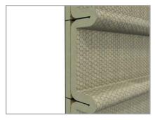
Example of A60 class solution for steel bulkhead with PAROC Marine Wired Mat 100. Insulating thickness on bulkhead is 40+40 mm and on stiffeners 40 mm.
