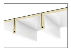
Example of A60 class solution for steel deck with PAROC Marine Fire Slab 100 G1 and preformed block PAROC Marine Fire Slab 100 G1, HPL. Insulating thickness on deck is 40 mm and on stiffener 25 mm.
