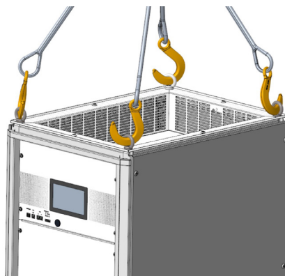
Figure 3: Transport of an cabinet SVGm by crane.
