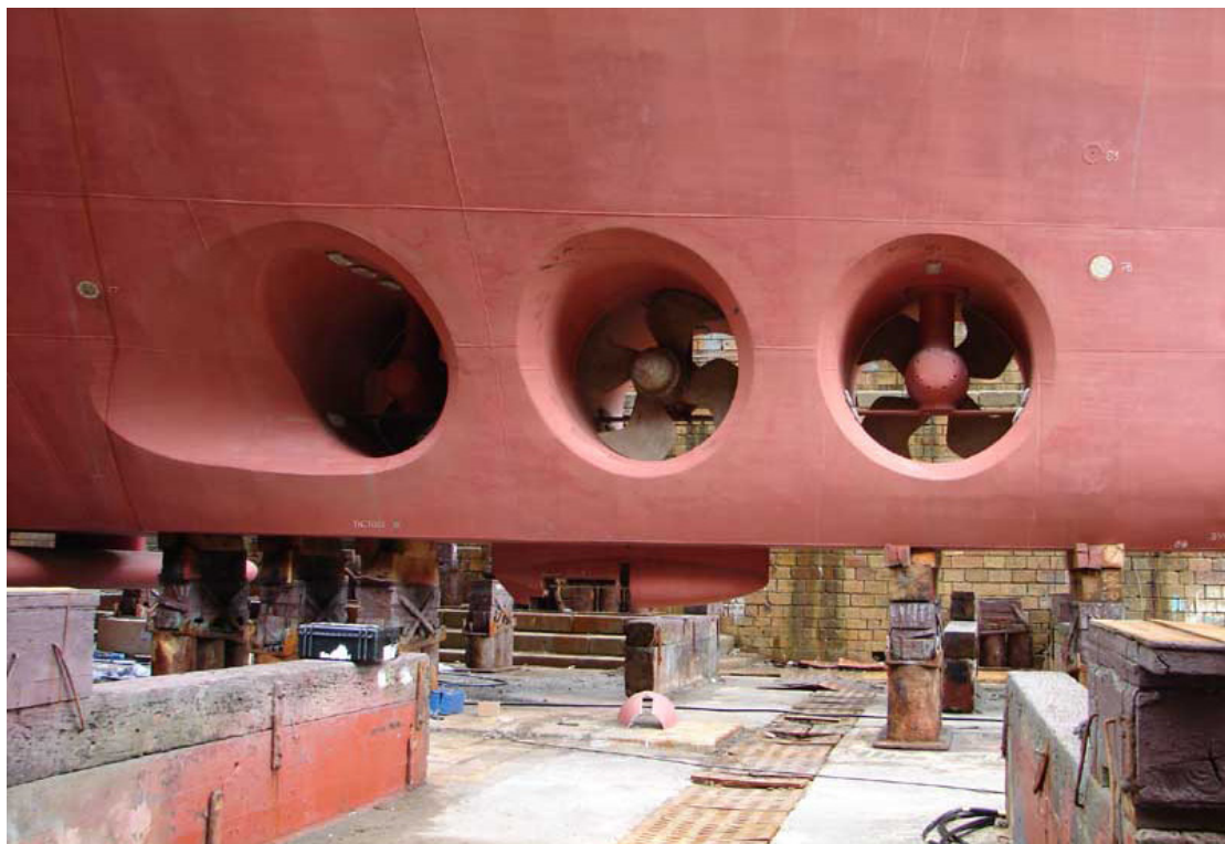
Application example: Soft starters are frequently selected for control of ship bow thrusters due to the large size of the motors relative to the generator.
