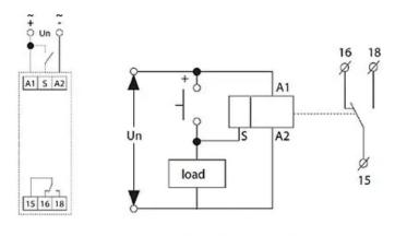
Connect control input to load
