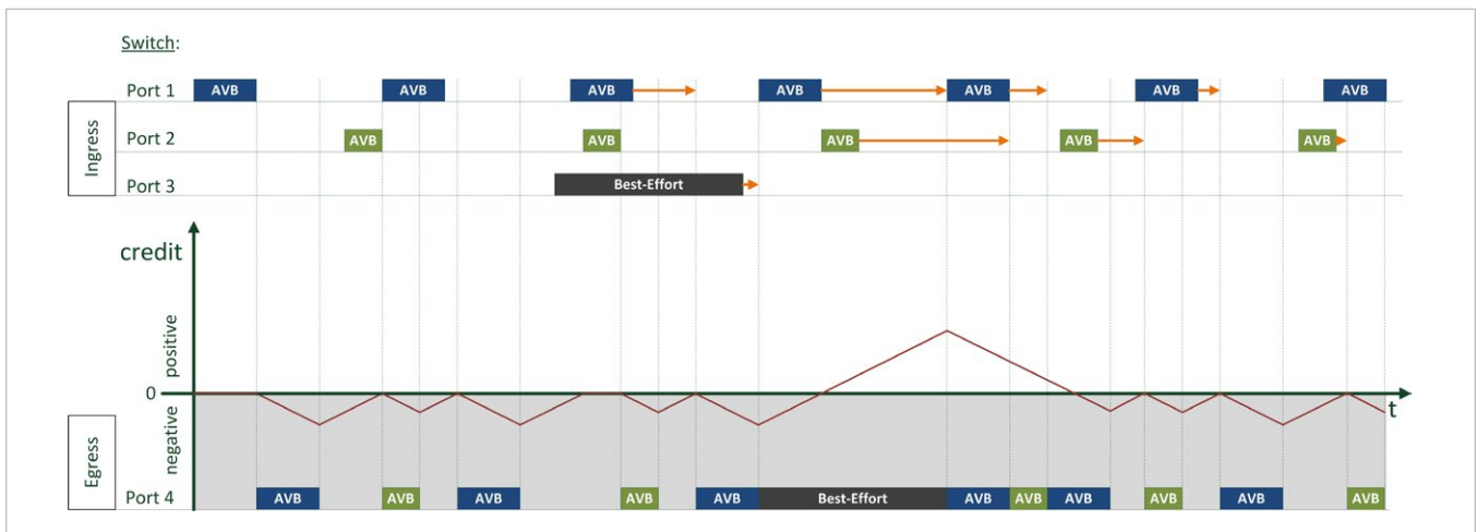
Figure 7: With the Credit-Based Shaper, data streams with reserved bandwidths are handled with higher priority than best effort traffic, as long as positive transmission credit is available
