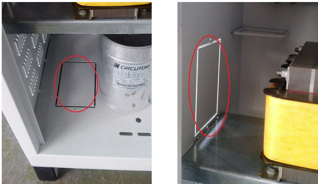
Figure 5: Cable entry points of the OPTIM FRES models.
