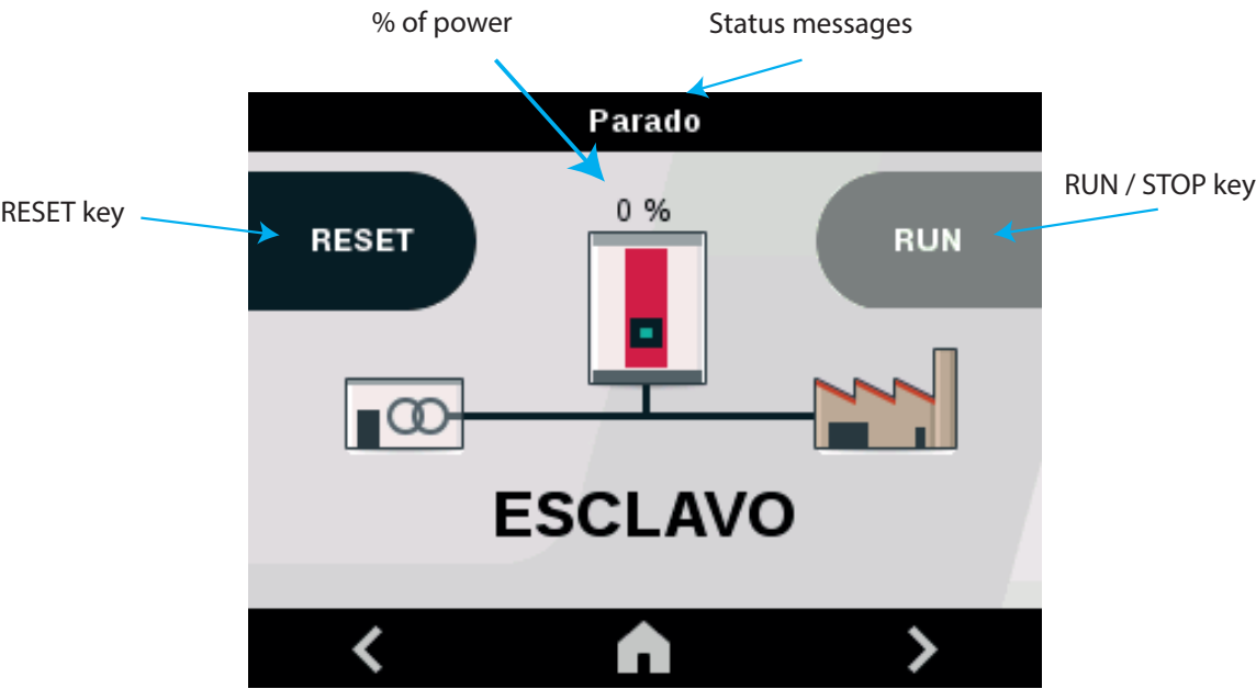
Figure 41: Main screen of the slave device.
