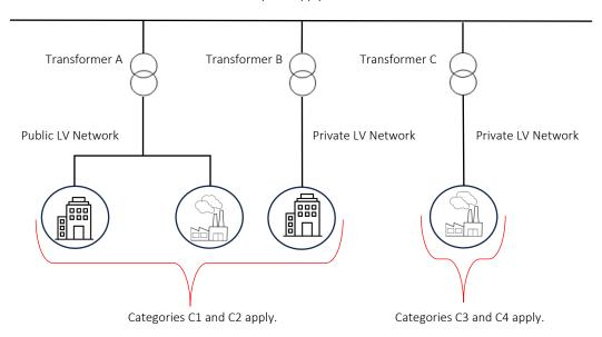
Transformer A supplies the public 415Vac LV network – First Environment. Transformer B supplies a private 415Vac LV network – considered First Environment. Transformer C supplies a private 415vac LV industrial network – Second Environment.
