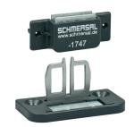
Note: The opening and closing functions depend on the direction of actuation, the actuating magnets and the polarity of the actuating magnets. | When the switches and actuators come together, the colours must coincide: Red (S) to red (S) and green (N) to green (N). This does not apply to the bistable contact. | The switch is to be mounted on iron with a non-magnetic layer of at least 20 mm.
