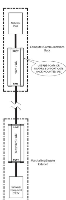
The EC90 version of this SPD has an isolated earth connection and it is recommended that this is installed at the field end of the cable run in conjunction with a standard unit at the network switch/controlling end of the cable. This will eliminate any earth loop issues when screened cable is used.
