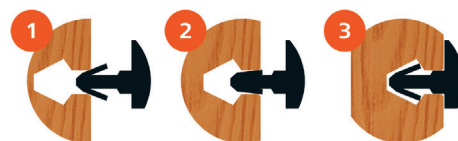
The boards simply click into place when depressed.
