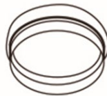
Round fitting for window unit, to be positioned between the end of the tube and the window unit itself
